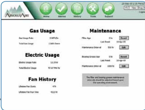
**Tools.** Maintenance intervals can be customized using the edit functions. When the filter age or bearing grease age exceeds its pre-set service interval, an alarm is activated.
