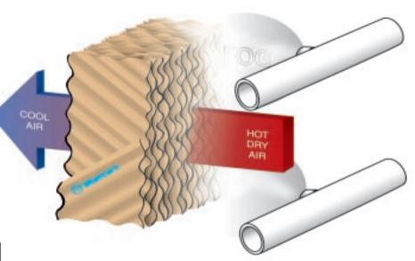
The steep angle of the flutes enhances the self-cleaning quality of MI-T-Fog by allowing water to continually flush dirt and debris from the face of the pad.
