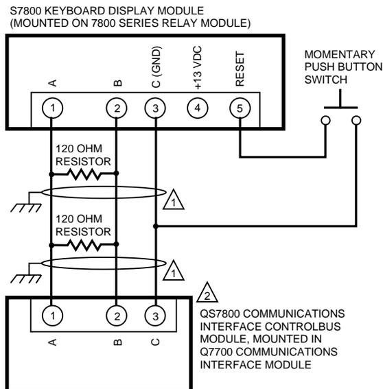
1 THREE WIRE SHIELDED CABLE MAY BE REQUIRED. TWO 120 OHM TERMINATING RESISTORS ARE REQUIRED FOR CONNECTIONS OVER 100 FEET (30 METERS). CABLE SHIELD MUST BE TERMINATED TO EARTH GROUND AT BOTH ENDS. IF SHIELDED CABLE IS NOT USED, TWISTED PAIR WIRE MUST BE USED.
