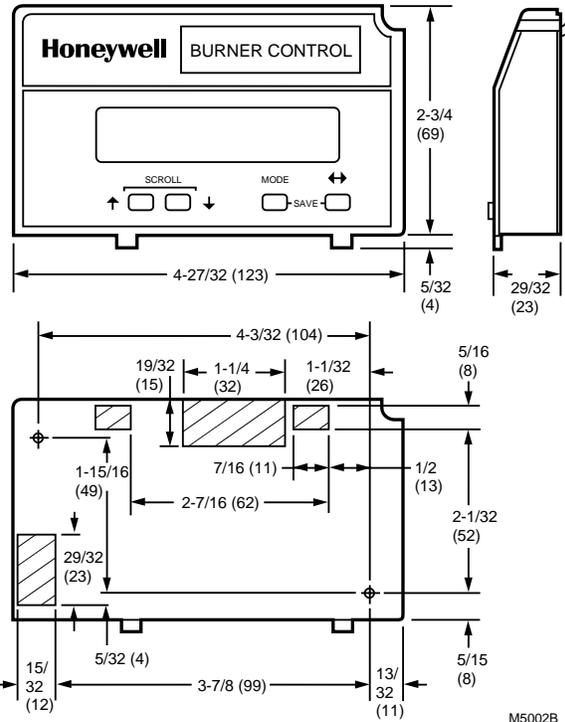
Fig. 1. Approximate dimensions of S7800 in in. (mm).
