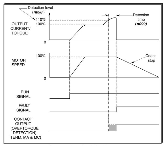
**Overtorque Detection Timing Diagram**
