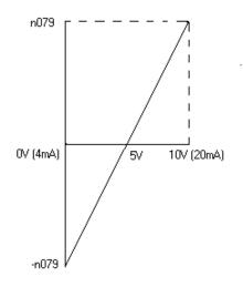
FBIAS is added to the frequency reference, after frequency reference gain (n060 (terminal FR) or n074 (terminal RP)) and frequency reference bias (n061 (terminal FR) or n075 (terminal RP)) are used to calculate master speed reference input at terminals FR or RP
