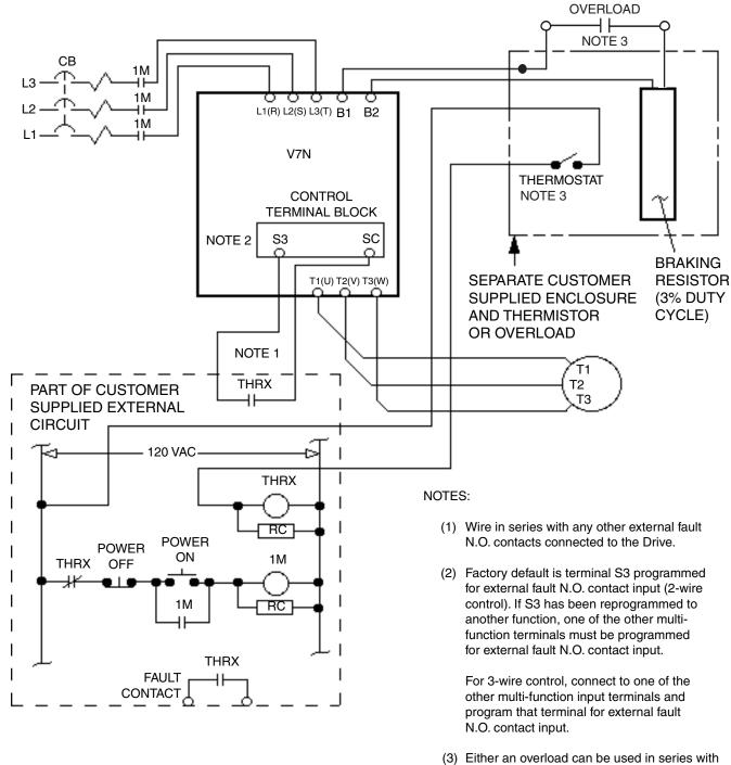
the Braking resistor or a thermostat can be configured as shown.
