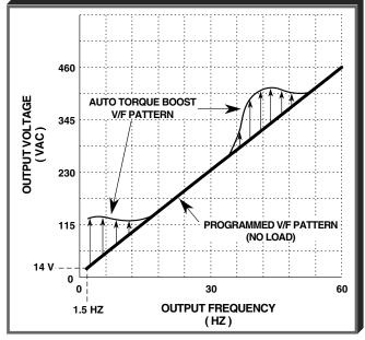
Example of Torque Compensation Operation
