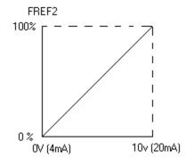
When multi-function analog input (n004 = 7 or 8) is selected, 2CN on the digital operator becomes the speed reference input. If n004 is set to any other data value, the 2CN auxiliary analog input is determined by the selection of Command A.
