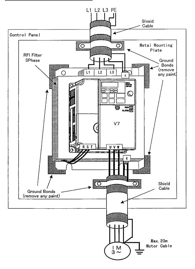
Figure 1-4. Installation of Line Filter and V7 Drive
