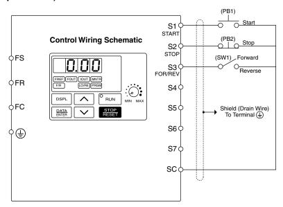
This configuration is best when a person rather than an external controller (PLC, relay, etc.) controls the drive.
