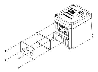
To remove the front cover of V74X [NEMA type 4X/12], models 25P5, 27P5, 45P5 and 47P5: Remove the six mounting bolts from the front of the enclosure, then carefully remove front cover.
