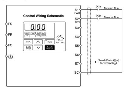
This configuration is used when the sequence comes from a remote source, such as a relay or a PLC. It can also be used with a maintained switch when it is desirable to have the drive restart on restoration of power. It should not be used where safety of attending personnel might be threatened by a restart.
