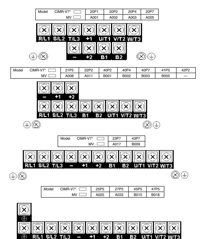
Figure 1-1c. Main Circuit Terminals
