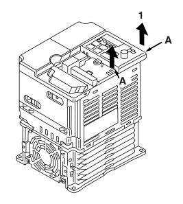
Removing bottom cover when "W"
