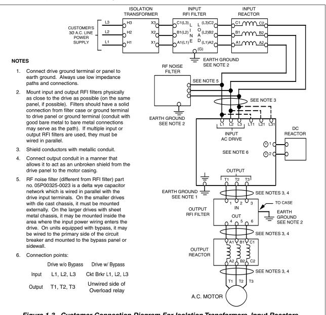
Figure 1-3. Customer Connection Diagram For Isolation Transformers, Input Reactors, Input RFI Filters, DC Reactors, Output Reactors and Output RFI Filters
