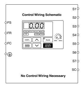
When the drive is set up with the sequence and the reference coming from the digital operator, it is in "Local" control. Local control is often used during startup to verify motor operation, rotation, etc. The drive can be temporarily placed in "Local" control simply by using the LO/RE quick start LED. If power is removed and then restored, the drive will come up in the "Remote" mode.
