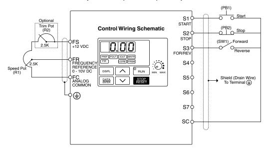
This configuration is best when a person rather than an external controller (PLC, relay, etc.) controls the drive. Both potentiometers ((R1) & (R2)) should have a resistance value between  $2000\Omega$  and  $3000\Omega$  and be rated for at least 1 Watt. The trim pot is optional, but without it the manual speed pot will output 10V (60 Hz) at just three-quarters of its rotation.
