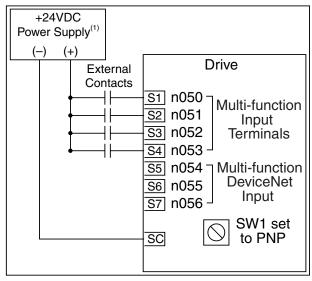
External wiring for PNP inputs
