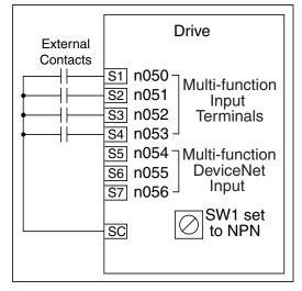
External wiring for NPN inputs
