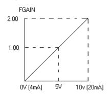
Frequency reference is multiplied by FGAIN, after frequency reference gain (n060 (terminal FR)) or n074 (terminal RP)) and frequency reference bias (n061 (terminal FR)) or n074 (terminal RP)) are used to calculate a master speed reference input at terminals FR or RP
