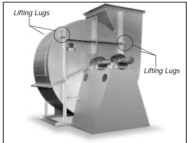
Housing should be lifted using straps and spreaders. Do not distort housing or side plates when lifting.
