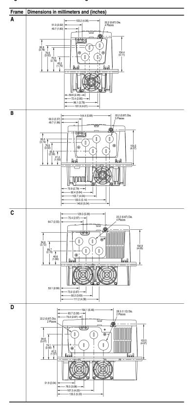
Figure 1.4 PowerFlex 70 Flange Mount Bottom View Dimensions
