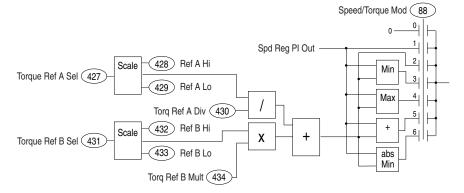
As shown, [Speed/Torque Mod] (parameter 88) is used to select the mode of operation. Zero torque current is allowed when set to "0."
