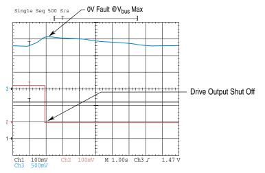
With bus regulation enabled, the drive can respond to the increasing voltage by advancing the output frequency until the regeneration is counteracted. This keeps the bus voltage at a regulated level below the trip point.
