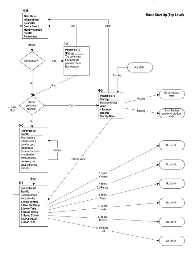
Figure 2.39 PowerFlex 70 & 700 Standard Control Option Startup
