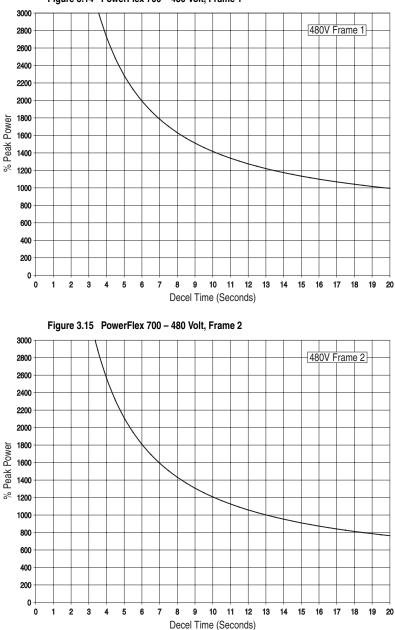
Figure 3.14 PowerFlex 700 - 480 Volt, Frame 1
