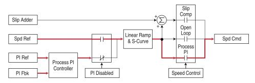
When the PI is enabled, the speed reference is disconnected and PI Output has exclusive control of the commanded speed, passing through the linear ramp and s-curve.
