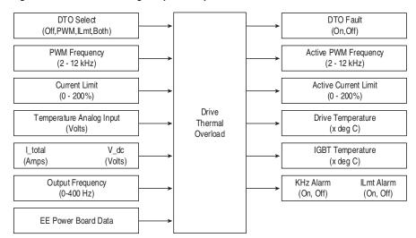
Figure 2.20 Thermal Manager Inputs/Outputs
