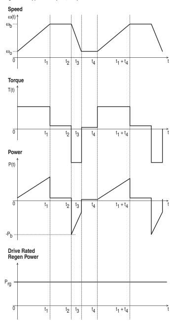
Figure 2.1 Application Speed, Torque and Power Profiles
