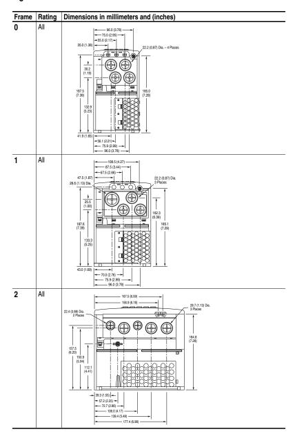
Figure 1.11 PowerFlex 700 Bottom View Dimensions
