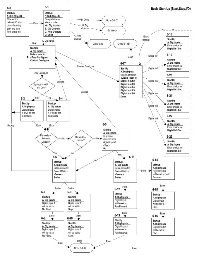
Figure 2.39 PowerFlex 70 & 700 Standard Control Option Startup (6)
