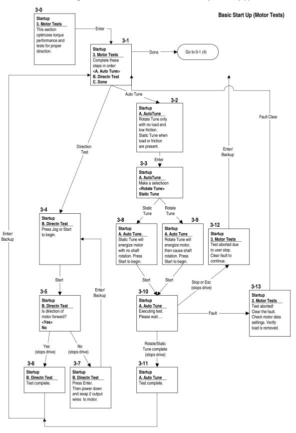
Figure 2.39 PowerFlex 70 & 700 Standard Control Option Startup (3)
