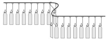
By programming the Shear Pin feature, the user can cause the drive to fault, stopping the excess torque before mechanical damage occurs.
