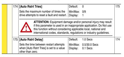
Setting [Auto Rstrt Tries] to a value greater than zero will enable the Auto Restart feature. Setting the number of tries equal to zero will disable the feature.
