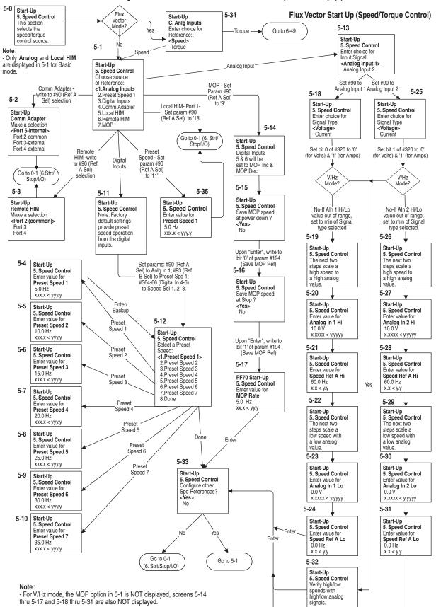
Figure 2.40 PowerFlex 700 Vector Control Option Startup (5)
