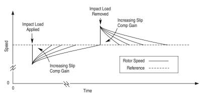
Figure 2.33 Rotor Speed Response Due to Impact Load and Slip Com Gain
