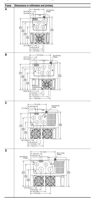
Figure 1.2 PowerFlex 70 IP20/NEMA Type 1 Bottom View Dimensions
