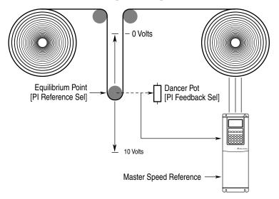
When the PI is disabled the commanded speed is the ramped speed reference.
