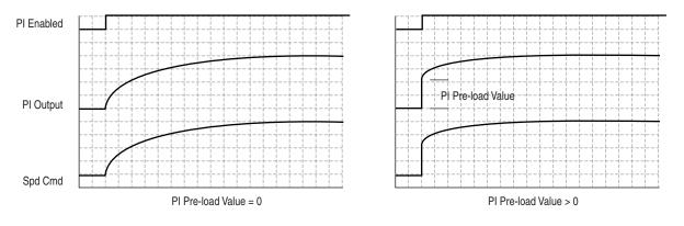
Pre-load command may be used when the PI has exclusive control of the commanded speed. With the integrator preset to the commanded speed there is no disturbance in commanded speed when PI is enabled. After PI is enabled the PI output is regulated to the required level.
