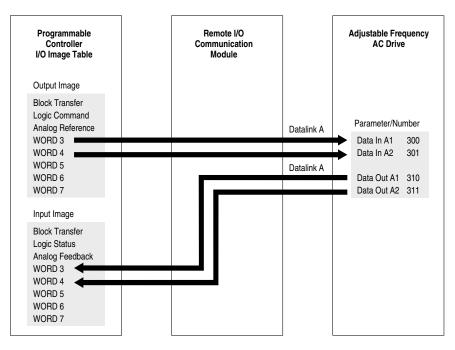
In the PLC data Table, the user enters Word 3 as a value of 100 (10.0 Secs) and word 4 as a value of 133 (13.3 seconds). On each I/O scan, the parameters in the PowerFlex drive are updated with the value from the data table:
