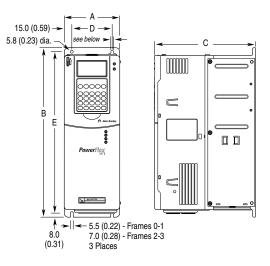
Dimensions are in millimeters and (inches)
