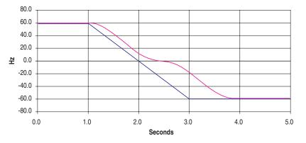
The following graph shows an acceleration time of 1.0 second. After 0.75 seconds, the acceleration time is changed to 6.0 seconds. When the acceleration rate is changed, the commanded rate is reduced to match the requested rate based on the initial S-curve calculation. After reaching the new acceleration rate, the S-curve is then changed to be a function of the new acceleration rate.
