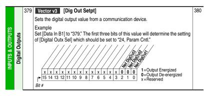
Example Digital Output 2 controlled by Data In B1
