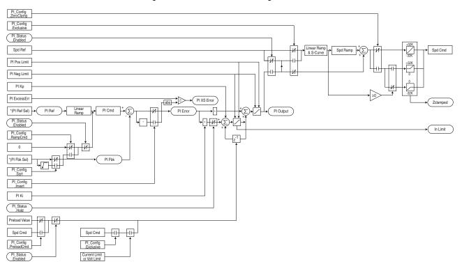
Figure 2.28 Process PI Block Diagram
