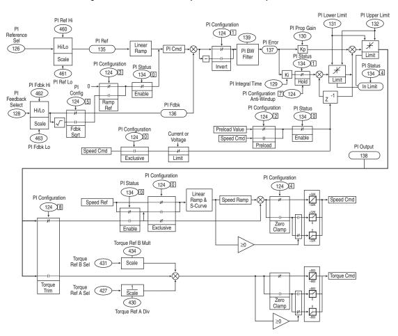
Figure 2.29 Vector Control Option Process PI Loop Overview
