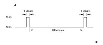
The ratio of 1:20 is the same for all durations of 150%. When operating continuous at 100%, if the load increases to 150% for 1 second the load must then return to 100% for 20 seconds before another step to 150%
