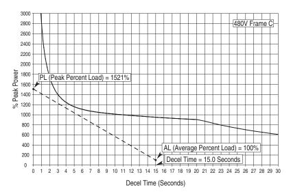
Figure 3.1 Example of an Acceptable Resistor Power Curve
