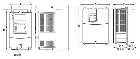
Dimensions are in millimeters and (inches).
