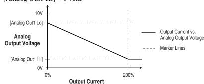
This example shows that you can have [Analog Out1 Lo] greater than [Analog Out1 Hi]. The result is a negative slope on the scaling from original quantity to analog output voltage. Negative slope could also be applied to any of the other examples in this section.
