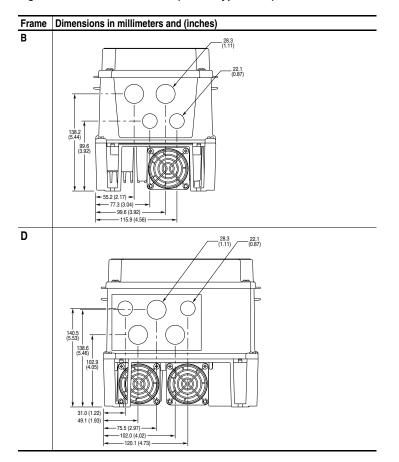
Figure 1.3 PowerFlex 70 IP66 (NEMA Type 4X/12) Bottom View Dimensions
