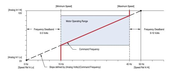
The deadband, as it relates to the analog input, can be calculated as follows:
