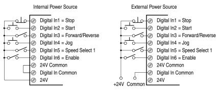
Figure 2.17 represents a typical digital input configuration that includes "2-wire" start. The digital input configuration parameters should be set up as shown
