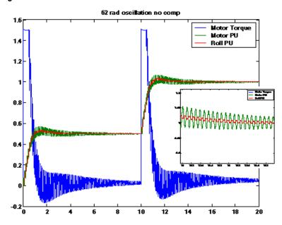
The insert shows the resonant frequency in detail.
