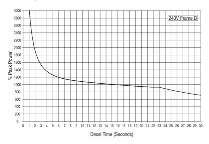
Figure 3.4 PowerFlex 70 - 240 Volt, Frame D
