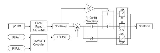
• Feedback Square Root - This feature uses the square root of the feedback signal as the PI feedback. This is useful in processes that control pressure, since centrifugal fans and pumps vary pressure with the square of speed.
