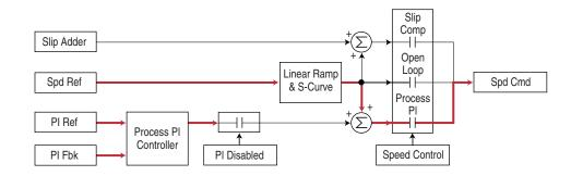
When the PI is enabled, the output of the PI Controller is added to the ramped speed reference.
