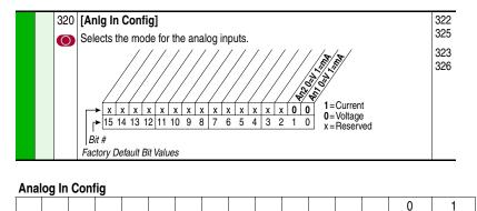
The input is scaled for 4-20 mA by setting [Analog In 1 Lo] to "4" mA and [Analog In 1 Hi] to "20" mA.
