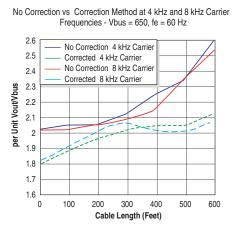
Without the correction, the overvoltage increases to unsafe levels with increasing cable length for both carrier frequencies.
