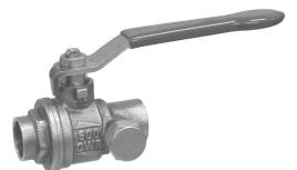
Solder End Series 481T valves are available in 1/2" and 3/4" (DN 15 and 20) sizes. Valves feature hex head side drain. When valve is in the closed position, the non-pressure side may be drained.
