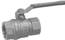
Threaded Series 451T and 456T are versatile generalpurpose valves from Jamesbury. Approvals for 451T are listed in Bulletin T110-1. Series 456T feature 316 stainless steel ball and stem which is a natural for saturated steam service to 150 psi (10.34 bar).
