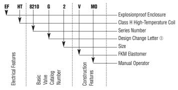
① The Design Change Letter indicates a major design change affecting spare parts kits, rebuild kits, and coils. The correct replacement parts for each change letter are shown in ASCO's Rebuild Kits and Coils Catalon
