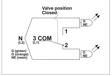
**Visual Indicator** Indicates closed and open position of the safety valve.
