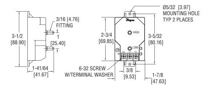
Our low cost Series 668 Differential Pressure Transmitter is capable of measuring low pressures with a  $\pm 1\%$  accuracy ideally suited for proper building pressurization and air flow control. Transmitters can withstand up to 10 psig overpressure with no damage to the unit. Variable capacitance sensor design provides excellent sensitivity and long-term stability. Compact, lightweight design makes installation simple and easy. Units also feature reverse-polarity protection.
