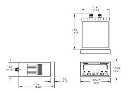
Face Designed to Meet NEMA 4X (IP66)
