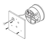
**B. SURFACE MOUNTING:** Drill (3) 3/16" dia. holes for mounting screws and (1) 7/8" dia. hole for wire assembly as shown in hole location drawing. Insert screws from rear of panel and thread into tapped holes on back of Photohelic® case. If rear pressure connections are to be used, make 1/2" dia. holes located as shown in hole location drawing in left column.
