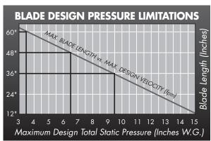
Series 1000 dampers exceeding the maximum design pressure due to blade length may be used by reducing the width of the damper sections and/or by increasing the number of sections per damper to maintain a blade width compatible with the required system pressure. (Example: 1 section damper of 60"w X 36"h (1525mm x 914mm) at 5" (1.24kPa) w.g. would need to be built in 2 sections of 30"w X 36"h (762mm x 914mm).)
