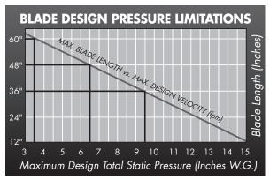
Series 1500 dampers exceeding the maximum design pressure due to blade length may be used by reducing the width of the damper sections and/or by increasing the number of sections per damper to maintain a blade width compatible with the required system pressure. (Example: 1 section damper of 60" w X 36" h (1525mm x 914mm) at 5" (1.24kPa) w.g. would need to be built in 2 sections of 30" w X 36" h (762mm x 914mm).)
