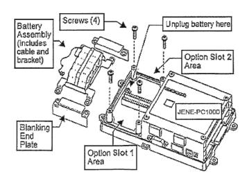
Remove the battery assembly (as shown) on the JENEsys™ PC1000 to install the JENE-PCLCD.
