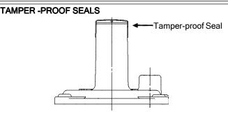
Permanent pressure sensitive backed paper. Attempted removal of these seals will destroy the face stock, leave adhesive residue on surface beneath, thus tampering can be easily detected. Available for all threaded models. Outlet pressure printed on seal.
